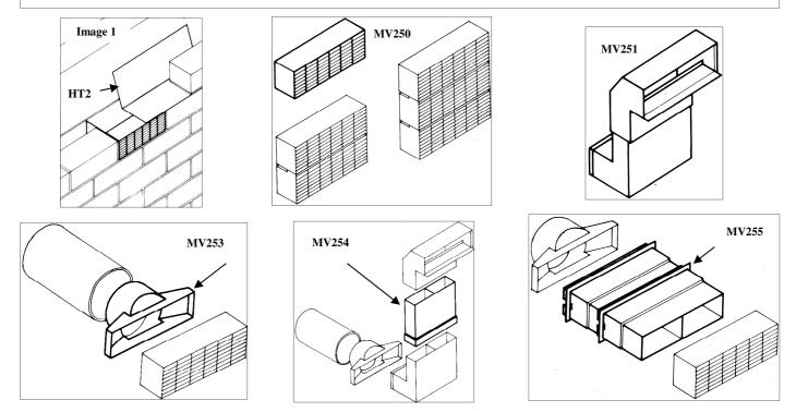
**MV250 AIRBRICK** (Pack quantity: 20). The Airbrick has an airflow of 8,000mm<sup>2</sup> and should be installed at a maximum of 2m centres. To provide a greater airflow it is possible to clip together a number of Airbricks in a vertical stack. The Airbrick can be used in combination with the Straight Sleeve, Vent Pipe Adaptor or Periscope. Three colours are available – buff, terracotta and anthracite.
